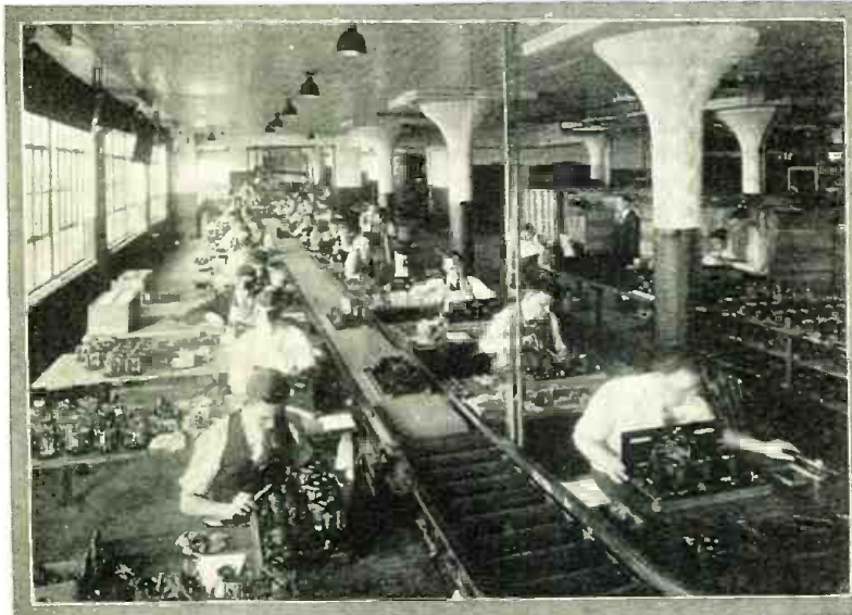
Above is shown the final assembly of the sets, with the operators who wire them. Belt-conveyor systems are used throughout the plant; and a section is here shown, carrying the sets from the workers.
